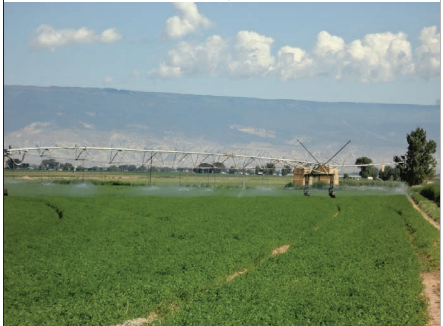
Figure 3: Center Pivot Sprinkler Irrigation in Montrose, Colorado
