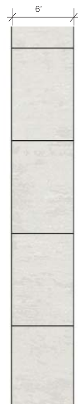
B Secondary Walk New Concrete with Sawcut Joints
