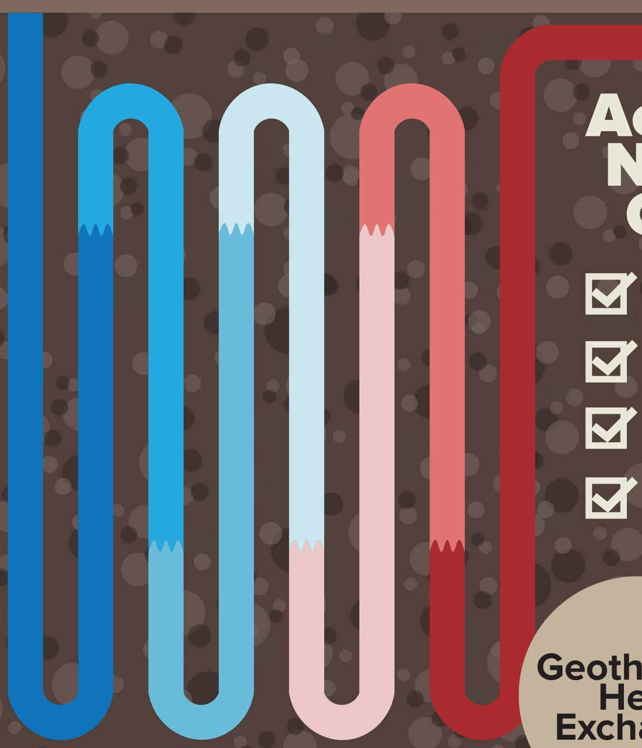
80 geothermal boreholes were drilled 400ft deep under the Armstrong Quad to circulate water to and from the library. During the cooling season, heat is expelled from the building and stored in the ground or sent to other buildings on campus. In the heating season, the library draws on that stored heat and existing geothermal heat to efficiently warm Tutt Library.
