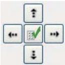
It is for OSD menu. You can select the any OSD menu using the arrow button. If the menu is open, you could not use Control function buttons.
