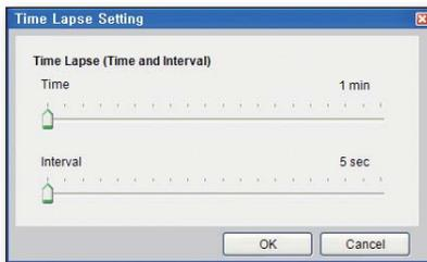
Time Lapse sets the frame rate for recording. If you set the "Interval" to 5 sec, you can get only 1 frame image for 5 sec interval. The result will look like high speed recording. You can apply limit to the total recording time. (The playback frame rate of Time Lapse recording will be fixed to 15frame/sec.)
