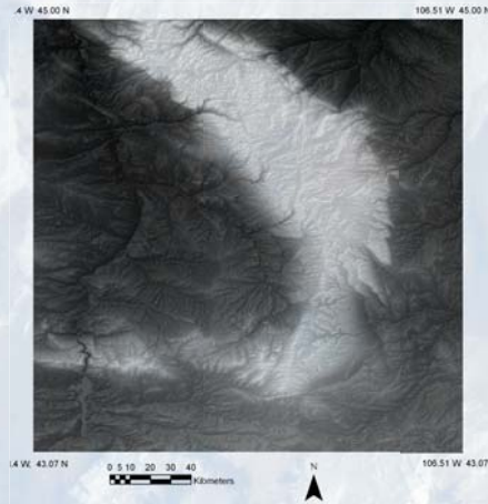
FIGURE 2. Shaded relief digital elevation model of the Bighorn Mountains, Wyoming. The white area corresponds to the elevated terrain that approximately corresponds to the crest of the elongate NW-SE-orientated structural arch.
