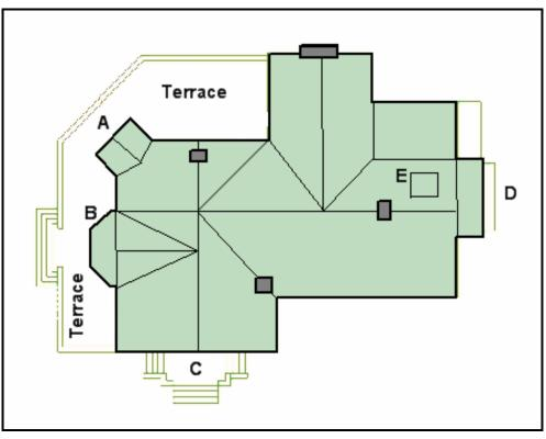
Figure 1. Plan view of Edgeplain showing roof planes, with chimneys indicated by darker rectangles on roof. North is to the right. Letters indicate selected features as follows: A, two-story bay window on southwest; B, two-story bay window on south; C, steps to front porch; D, one-story porch on north; and E, shed roof dormer.
