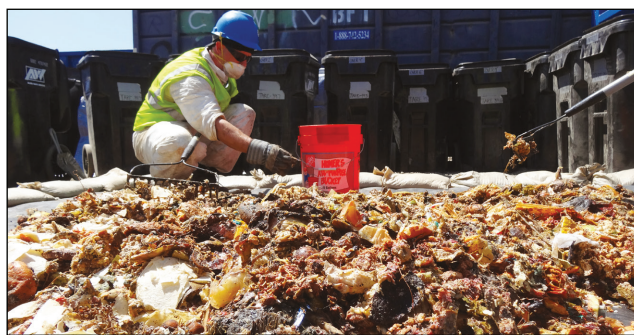
Figure 1. Sorting food waste is dirty work but is important for estimating greenhouse-gas emissions from landfills. In this study by Eugene Tsang at the Sunshine Canyon Landfill in Los Angeles, sorted food waste is separated to undergo methane production analysis.
