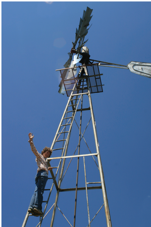
Wind turbine used to pump water for cattle at Fort Union
