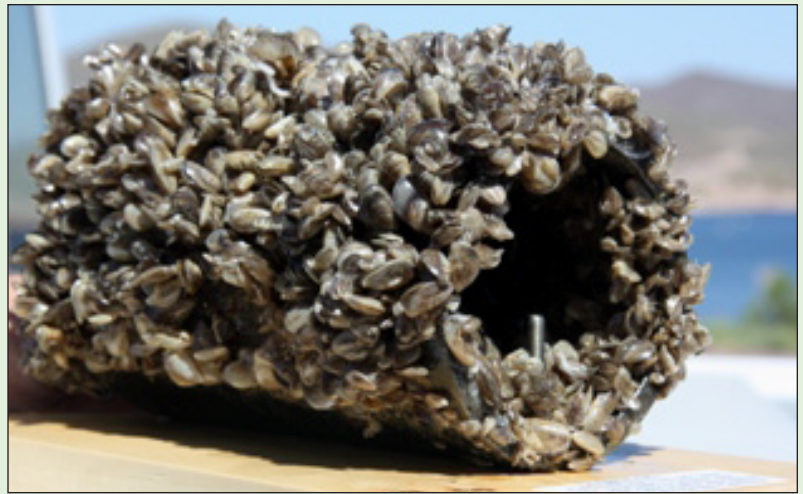
Figure 16: Quagga Colony on Pipe
